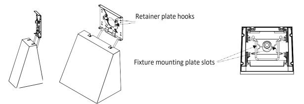
6. Secure the fixture to the wall mounting plate using the  $1/4''-20 \times 1$  hex socket cap screws (x 2), from step 1, and 3/16'' allen wrench.
