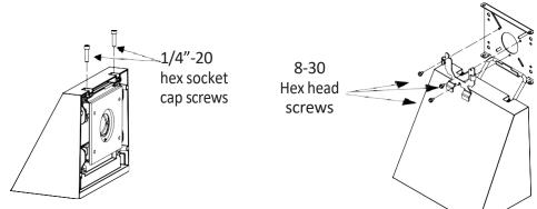
2. Position the wall mounting plate over the j-box. Attach the plate to the j-box using screws that came with the j-box. (see the chart on the next page for fixture weights)
