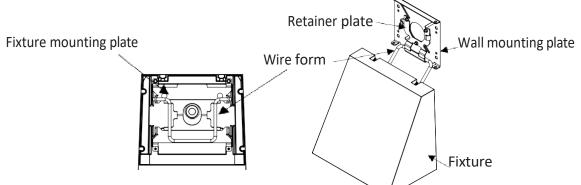
1. Use the 3/16'' allen wrench or hex key to detach the wall mounting plate from the fixture by removing the 1/4''-20 x 1 hex socket cap screws (x 2).
