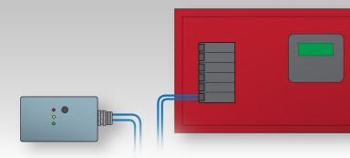
IOTA® ETS 20 and ETS 20 DR solutions allow the use of local controls on designated emergency lighting circuits, enabling users to turn multiple fixtures on or off or dim to desired levels without impacting their code-required emergency lighting function. During an emergency, the IOTA ETS 20 can bypass local controls or dim settings and cause the designated emergency fixtures to be powered at full light output for optimal occupant safety.
