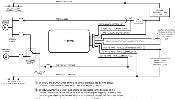
(3) Observe proper polarity, if necessary. No more than (5) ETS 20 units can be installed in parallel with a remote device.
