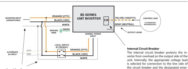
The IIS Inverter utilizes two sets of input leads: one to provide unswitched power to the inverter system and a second to serve as a normal power input to the lighting load. Any switch for the designated emergency circuit will be present on the Normal Power Input leads. For Emergency Operation Only applications, the Normal Input leads are not needed and would remain disconnected and capped.
