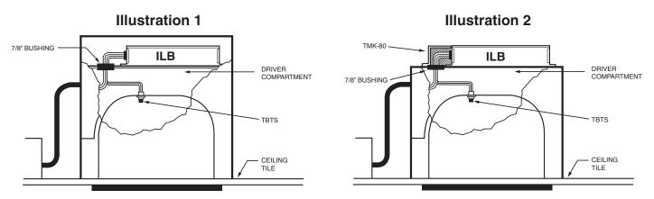
NOTE: Position the **TBTS** so that it can be seen after installation.
