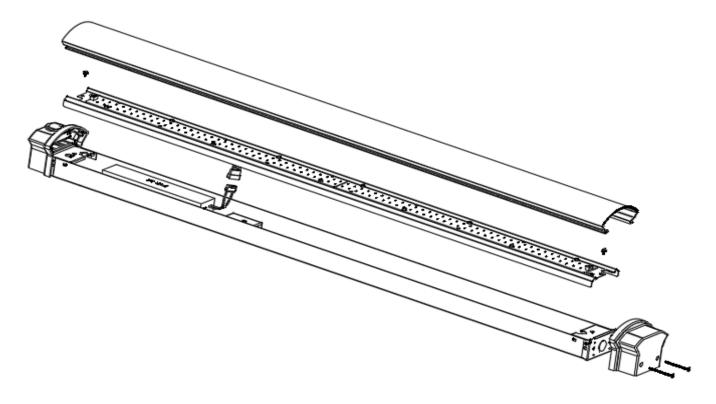
SEAT CHANNEL COVER ONTO HOUSING AND SECURE WITH THE (2) SCREWS.
