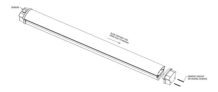
REMOVE THE TWO SCREWS THAT ARE SECURING THE CHANNEL COVER/BOARD ASSEMBLY.
