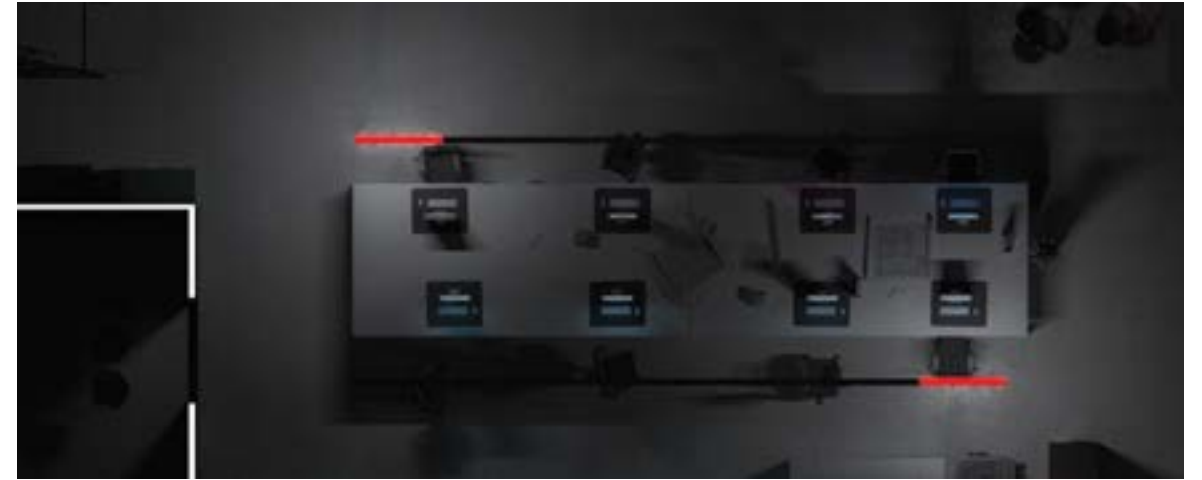
Traditional emergency layout that only lights the path of egress and exits from the building, which meet the minimum safety requirements.
