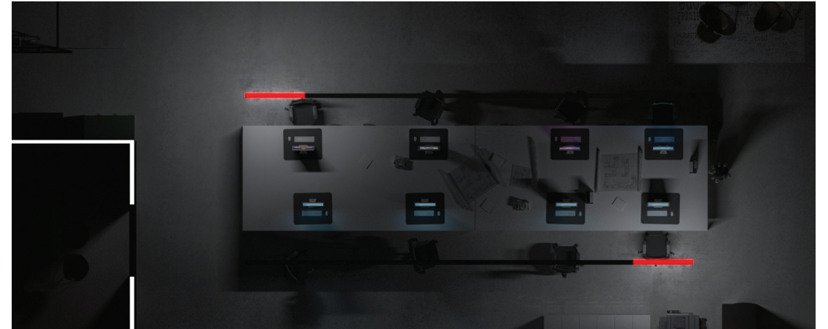
Integral driver emergency layout that only lights the path of egress and exits from the building, which meet the minimum safety requirements.
