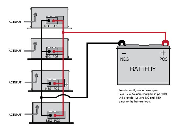
This illustration demonstrates a typical parallel configuration system. When the battery chargers are connected in parallel, the system delivers increased amperage (*amps x number of chargers*) with no effect on the output voltage.
