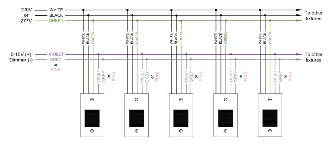
Note: For NON-DIMMING installations, cap violet and grey or pink wires separately. Do not cap together.
