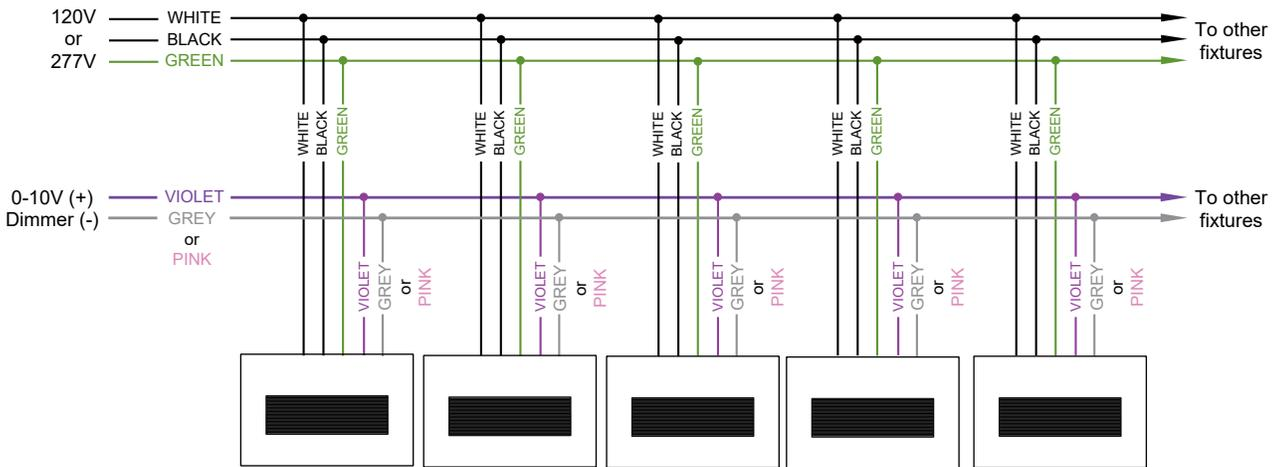
*Note: For NON-DIMMING installations, cap violet and grey or pink wires separately. Do not cap together.*
