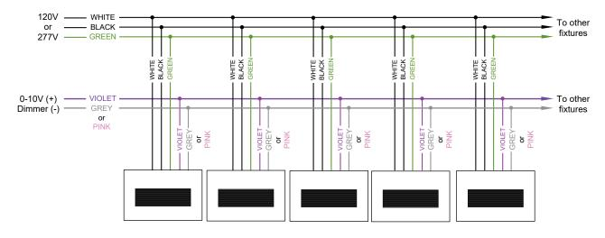
Note: For NON-DIMMING installations, cap violet and grey or pink wires separately. Do not cap together.
