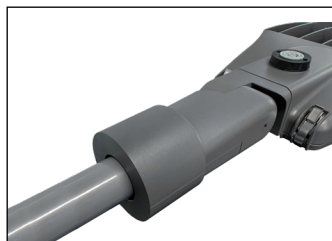
Vertical Tenon/Horizontal Arm Mount – VH Attaches to 2" vertical tenon or horizontal mast arm (2 3/8" O.D.)
