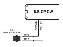
C. Connect the IPS White wire to the Brown lead on the ILB. Then connect the IPS Red wire to the Violet lead.
