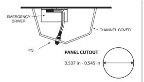
A. Locate a suitable location for the IPS and cable that is visible outside the fixture. Drill or punch a 0.537" diameter hole in the fixture wall or wireway cover. Insert the IPS into the hole so that the LED test button/pilot light is located outside of the fixture.
