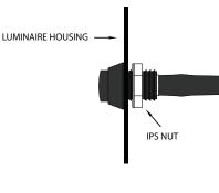
B. Secure the IPS using the IPS nut.
