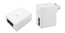
Power to a **nIO D / nIO 1S** device is provided by the CAT-5e connection to an nLight power pack/supply or other nLight device supplying bus power. If power is not present on the CAT-5e bus, the **nIO D**'s dimming output will release lights to highest level. T568B pin/pair assignment is recommended for all CAT-5e cables.
