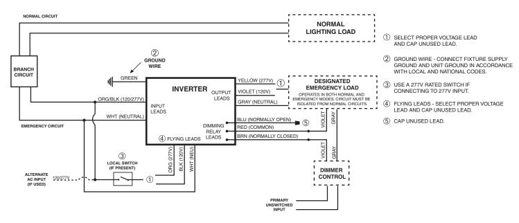
The Dimming Relay contacts provide electrical continuity during normal power conditions allowing your dimming signal to operate the luminaire in the desired, dimmed state. When the inverter transfers into the emergency mode, the dimming relay contacts electrically open the 0-10 dimming reference signal forcing the luminaire to operate at full lumen output regardless of dimmer setting.
