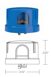
The DE Series photocontrol utilizes premium components, a silicon light sensor and an infrared blocking filter to provide human eye spectral response and consistent turn-on night after night, over the life of the control.
