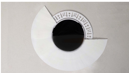
An IVO downlight requires only approximately 3" of plaster to finish.
