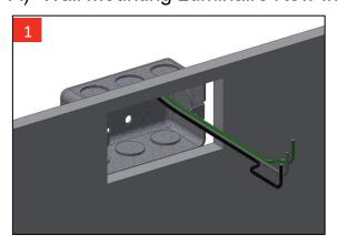
1. Using a laser or snap line, mark wall for center line. Using Support Spacing diagram determine locations of power feed and supports. Cut wall material for 2"x4" switch box at feed location. Pull building wires as shown.
