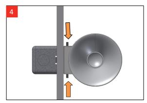
4. Hang the luminaire on the support bracket. Secure luminaire to each support bracket using (4) provided set screws and adjust level of luminaire where necessary.
