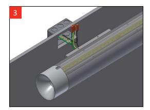
3. Raise the first luminaire into position. At power feed locations, connect building wires with fixture wires using appropriate twist-on connectors. Gently place wire connection back into luminaire and switch box.
