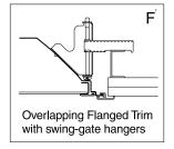
1 Recommended rough-in dimensions for F-trim fixtures 24"x24" (Tolerance is +1/4"-0"). Swing-gate range 1-3/16" to 3-15/16". Swing-gate span 23-3/8" to 26-11/16". Fixture swing-gate points require additional 1-1/16" over nominal fixture height.
