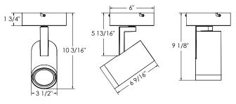
0-10V dimmable driver mounted in a deep canopy • 0-10V dimming requires two (2) additional low-voltage wires to be pulled. **Dimming** MVOLT versions are phase-dimmable (120V only) down to 10% or less using high quality, factory-approved dimmers - see <u>R600LG2-</u> <u>DIM</u> • MVOLT versions are also 0-10V dimmable down to as low as 1% and require two (2) additional low-voltage wires to be pulled • 347V
