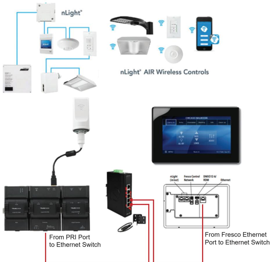
This is an example diagram for setting up an Eclipse with nLight Air, nLight Wired and Fresco devices. Each of these nLight devices will show up in Sensorview, Yabe, or a BACnet Client as BACnet points. These points are automatically created and have certain properties and settings associated with each.
