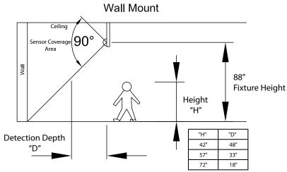
When wall mounted (such as above entry door), motion detection ("D") will be affected by height of person ("H"), and depth of room.
