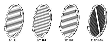
TKO optic kit includes a 5°, 10° and 15° tilt filters and a 5° axial spread filter. TKO kits are standard on PDX4 LED fixtures and include a mounting ring.
