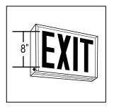
Letters 8" high with 1" stroke, with 100 ft viewing distance rating, based upon UL924 standards meets New York City requirements.
