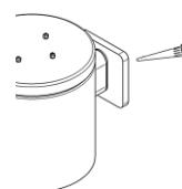
After mounting fixture to wall, place a bead of silicone-based caulking compound where the mounting brackets meets the wall on the top and on each side. Do NOT caulk along the bottom.
