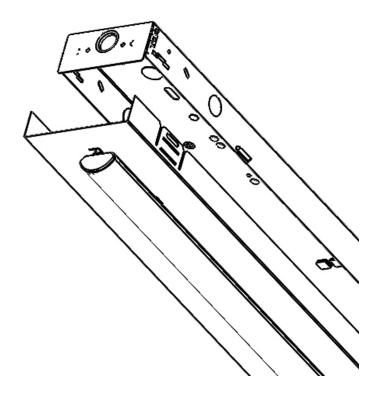
• Install using provided tek screws through mounting bracket, as shown. Note: A min torque of 20 in-lb needs to be applied to ensure secure assembly of kit to the housing.
