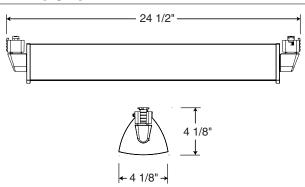
Alternate HTYPE Trac Adapter Compatible with track systems which use a H-type track adapter, including Lithonia LTS Decorative Track (not LT type) • System specific and assembled to trac fixture • Two-position power contact provided for two-circuit application • Consult factory for additional information.
