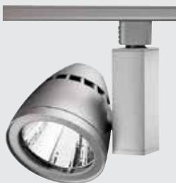
The elegant Conix II LED features durable, all-metal construction finished in lustrous white, black, or silver finishes. The fixture footprint is minimized by attaching the track head to a vertical, side-mount housing that contains the LED driver. With 360° rotation and more than 90° vertical aiming, these fixtures deliver extraordinary functionality. All wiring is fully concealed.
