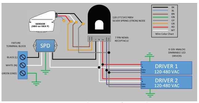
7-Pin NEMA Receptacle Wiring Diagram for 0-10V Analog Dimming
