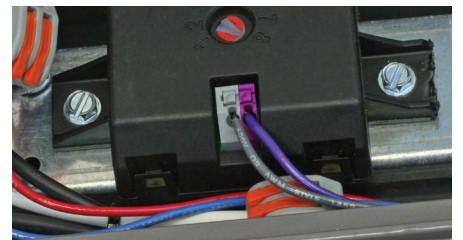
FAO module option for field-adjustable lumen output
