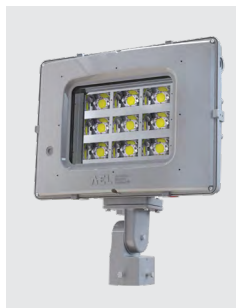
ACP2 LED Maximum weight: 80lbs. Yoke Maximum weight: 71lbs. Knuckle Maximum E.P.A.: 3.8 sq ft
