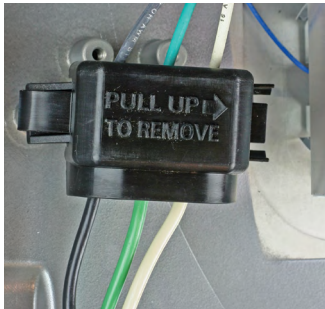
Prewired 3-stage terminal block for simplified installation
