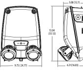
EXTL SP640L/ SP1100L/SP2200L Specifications Length: 10.42(26.47) Depth: 6.42(15.85) Height: 13.94(35.41) Weight of SP640L / SP1100L: 5.55lbs (2.52kg) Weight of LP2200L: 7.65 lbs (3.47kg)
