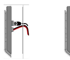
Pull all wires out of the wall and run them through the central hole of the backplate. Screw the backplate onto **• •** the wall.
