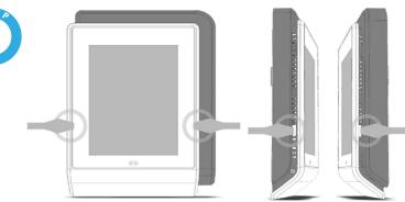
To mount, the faceplate must be detached from the backplate. This will require an appropriately sized tool (i.e., flat-head screwdriver) that can fit in the release tab.
