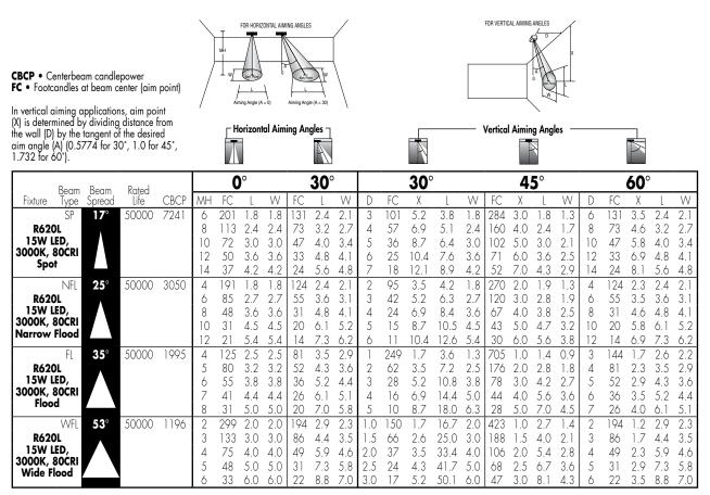
Also note that, due to the variable nature of the R620L optical system, beamspread types (shown above in table) are nominally chosen to represent typical designations found in dedicated beam designs - actual results, though comparable, may vary in the field.
